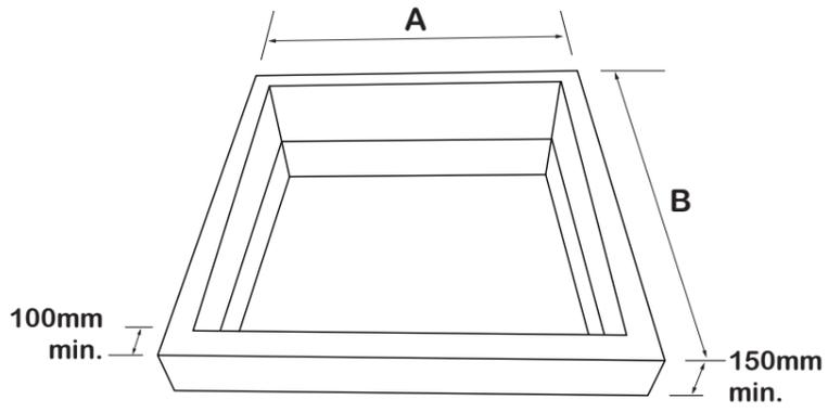
Skylight frame may be fitted before or after any roofing felt.
