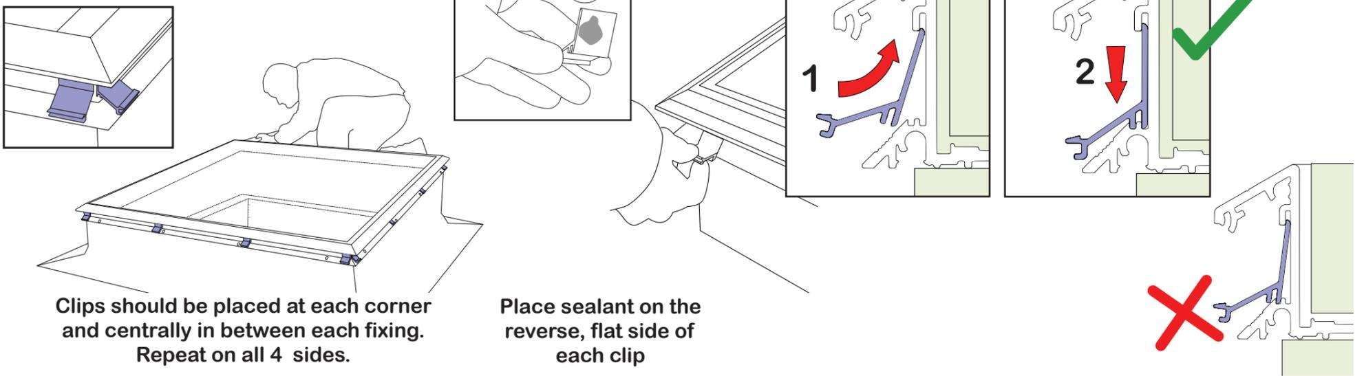
Clips should be placed at each corner and centrally in between each fixing. Repeat on all 4 sides.
